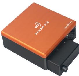
We've optimized the sample coupling optics of our integrated Raman systems to deliver a 50  $\mu\text{m}$  laser spot at a standard 25 mm working distance. Raman signal collection takes advantage of the spectrometer's full f/1.3 field of view for maximum sensitivity at the shortest acquisition times. An OD 6 laser rejection filter blocks unwanted scatter back into the system, passing Raman signal above ~200  $\text{cm}^{-1}$  (depending on excitation wavelength).
