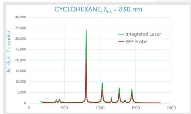
Use of high efficiency optics, careful filtering, and internal stray light management ensures that our integrated systems offer low background and noise, comparable to a matched NA probe/spectrometer system design. As can be seen above in a comparison of cyclohexane studied with 830 nm excitation, the integrated system outperforms a modular spectrometer/probe system in terms of signal level. This has tangible benefits in limit of detection.
