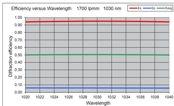
We measure every transmissive VPH grating to ensure exceptional 1<sup>st</sup> order diffractional efficiency. Many other vendors report only theoretical graphs of total diffraction efficiency. This includes diffraction into other orders, and is not truly representative of actual performance.
