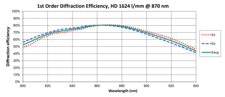
Diffraction efficiency curves are theoretical. Actual performance will vary slightly. Includes: glass absorption data, adhesive absorption data, film absorption data, manufacturing tolerances.
