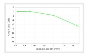
The Cobra VIS uses proprietary optics and a high sensitivity camera to deliver better roll-off than most OCT spectrometers, improving your resolution at increasing depths.
