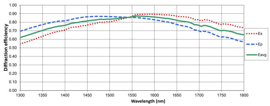
Diffraction efficiency curves are theoretical. Actual performance will vary slightly. Includes: glass absorption data, adhesive absorption data, film absorption data, manufacturing tolerances.
