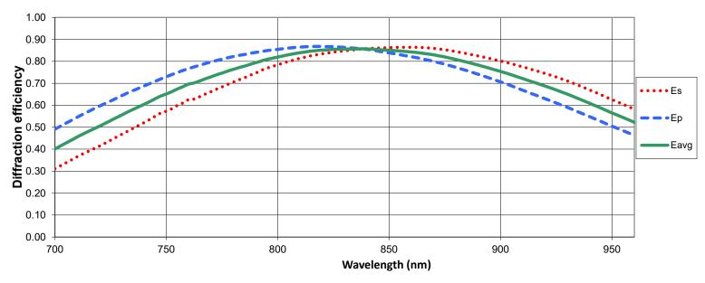
Diffraction efficiency curves are theoretical. Actual performance will vary slightly. Includes: glass absorption data, adhesive absorption data, film absorption data, manufacturing tolerances.
