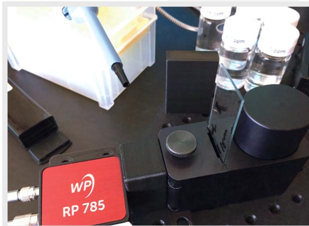
Figure 4: Wasatch Photonics Raman probe, spacer, and sample holder with Nikalyte SERS substrate inserted (left to right).
