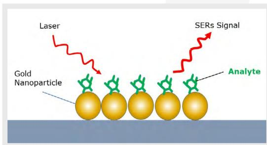
Figure 1: Surface Enhanced Raman Spectroscopy (SERS) using gold nanoparticles. (Image courtesy of [Nikalyte Ltd.](#))
