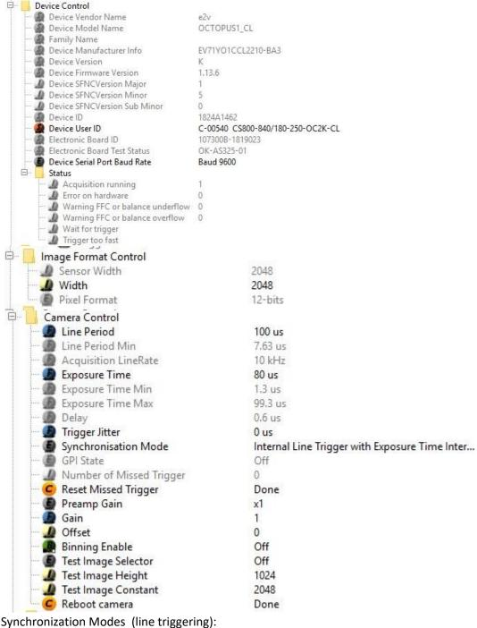
Internal Line Trigger with Exposure Time Internally controlled
