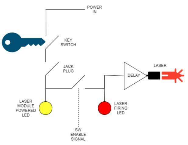
As can be seen from the diagram, the laser module has power when the System power supply is plugged in AND the key switch is engaged AND the jack plug contacts are connected together.
