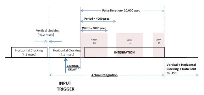
Four parameters define the above external trigger (laser) behavior. All parameters are independent of integration time and are enabled using the MOD\_ENABLE = 1 and SET LASER ENABLE = 1 commands illustrated in the example in Section 4.3.
