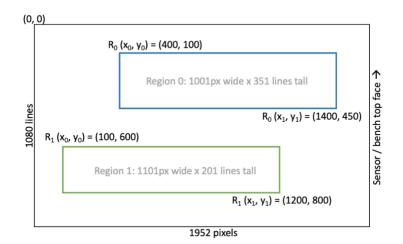
To configure the two ROIs ( $R_0$  and  $R_1$ ) on an IMX385 detector, you would send the following two SET\_DETECTOR\_ROI commands:
